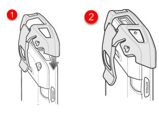
2. Removal: From the front of the carrying clip, push upward until it's removed.
